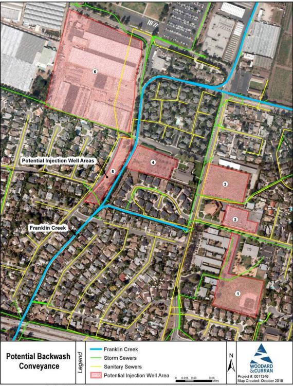
Figure 2-8: Potential Backwash Discharge Locations
