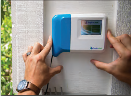
The user interface of Web-based smart irrigation controllers is much more understandable. Get one that can submeter water flow.
